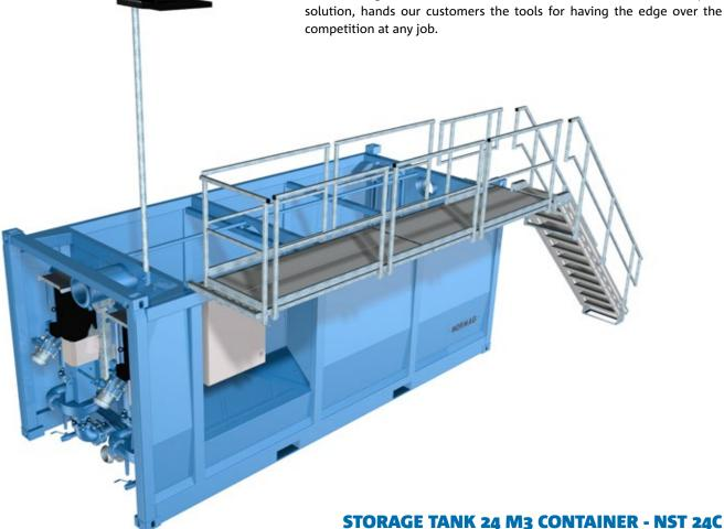
The 'Normag Storage Tank' serves practical use as additional active tank to feed the high pressure pump and simultaneously enlarges process volume for the drill and collects the excess cleaned mud of the reclaimer(s). It offers sufficiently installed power to provide pre-pressure for any high pressure pump and whilst keeping the active volume in suspension. Designed to interact with other Normag installations for autonomous operation, but also combines easily with other makes.
